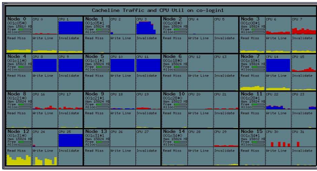
Fig. 2. A screen shot of the performance monitoring tool pmsub on SGI Altix. The light yellow area reflects how many remote memory accesses have occurred.
