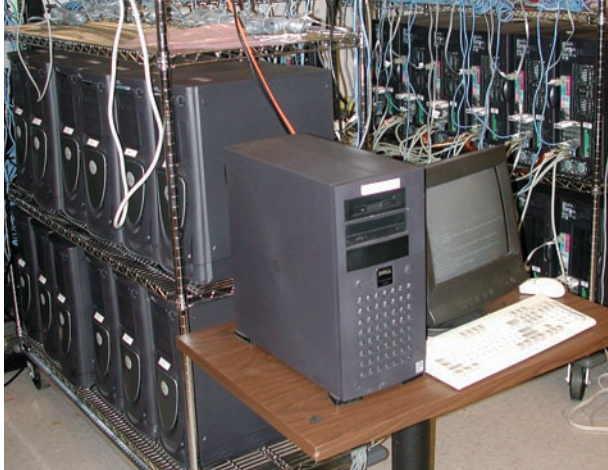
Cluster of 32 Dual P4 2.4 Ghz machines
